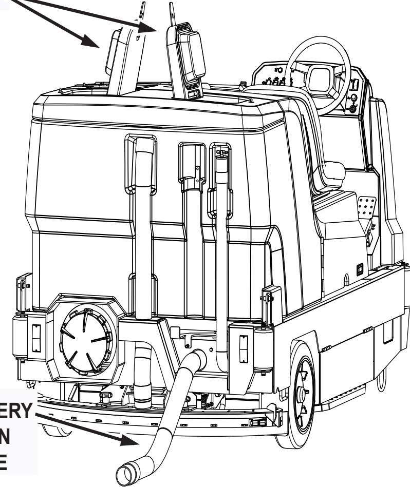
Fig. 1: Draining the Recovery Tank
